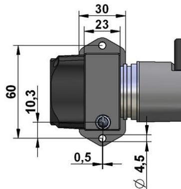
Detailed view: battery (data storage) integrated in the cable
