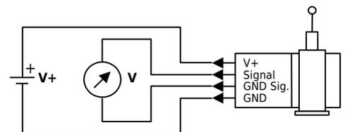
Note: GND Sig. and GND may be connected in a 3-wire system.
