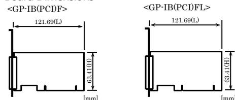
The standard outside dimension (L) is the distance from the end of the board to the outer surface of the slot cover.
