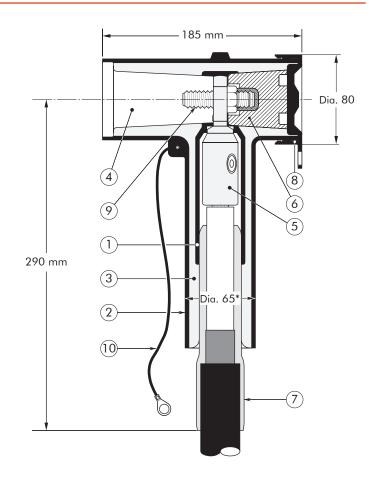
\* The indicated diameter is a die dimension. Depending on the conductor cross-section used, a deviation of up to + 5 mm is possible.
