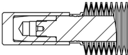
Using Item No. 1, push bellows over spigot until located in groove.
