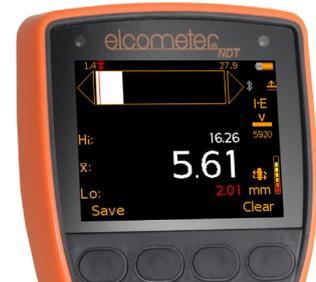
In scan mode the gauge takes readings at a rate of 16 Hz (16 readings per second).
