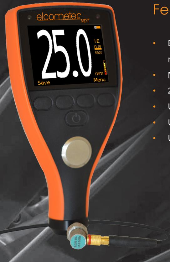
When precision is key, the PTG6 has a measurement range of 0.15mm(0.006") to 25mm (1.000") with  $\pm 1\%$  accuracy, across three measurement modes, Echo-Echo ThruPaint™, Interface Echo (I-E) and Plastic Mode (PLAS). This gauge allows users to take measurements with pinpoint accuracy.
